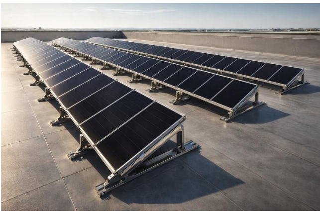
When choosing from the standard fixed “Jack Ready” mounts available, there is an additional option for a 15° vertical angle and 60 cm aisle width. Another advantage of the PV system with higher efficiency is that standard PV panel mounts, which Telab has been manufacturing in the Czech Republic for years and has Figure 7: “Jack Ready” mounts assembled facing south
